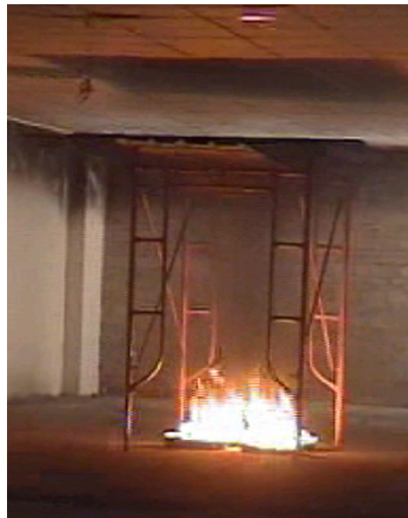
Fig. 2. Photo of the steel board above the fire during the full scale tests.
